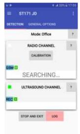
Establishing connection will be done in few seconds. «STATUS» indicator will change its indication to reverse one: permanent flashing is interrupted 1 time per second and «SEARCH» sign disappears. Also, in upper left corner of «RF blocker detection» section blinking green square will appear (similarly to «US blocker detection » section).
