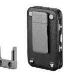
**Turning-on of the RM** is done by long press on turn-on button for around 5 seconds. When releasing «STATUS» indicator should flash one time per second. If indication is absent, battery should be charged.
