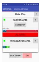
In **«ULTRASONIC CHANNEL»** window sonic and ultrasonic **«REC»** range, which is used by Dictaphone blockers, signals level is indicated.
