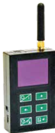
ST 165 Detector of wireless protocols
